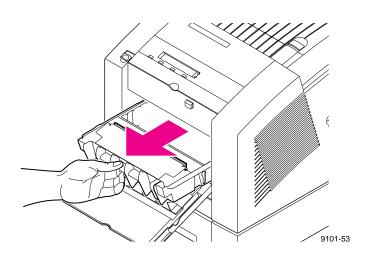
Note Once the maintenance tray has been partially used, it leaks drum fluid if tipped. Never ship a partially used maintenance tray.
